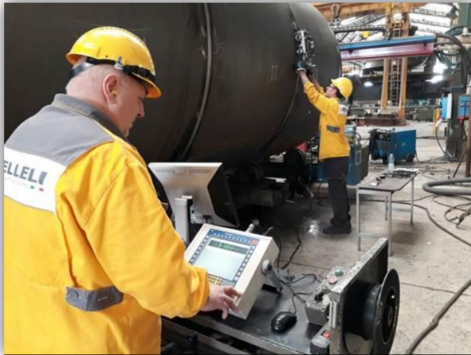
TEST AT FABRICATION SHOP (TOFD+PAUT)
