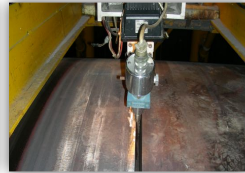
NARROW GAP & MONOWELD TECHNOLOGY
