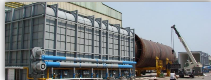
NOZZLE PREHEATING ARRANGEMENT (ELECTRICAL RESISTANCES + GAS BURNERS)
