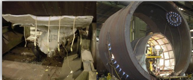
NOZZLE PREHEATING ARRANGEMENT (ELECTRICAL RESISTANCES + GAS BURNERS)
