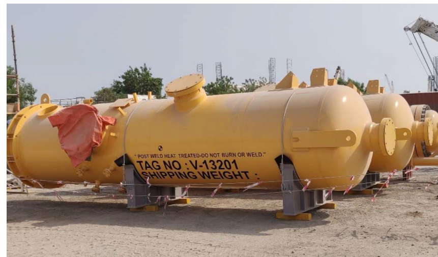
Dehydration Inlet Gas Scrubbers
