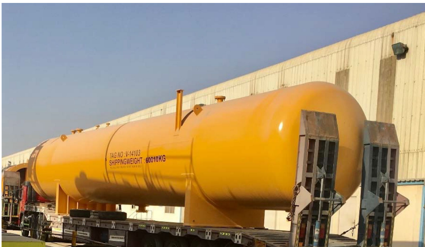
NGL Surge Tank
